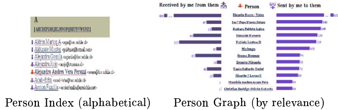
Fig. 1. Persons are shown in two indices. The person index (left) shows persons in alphabetical order, with icons representing their relative importance. The person graph (right) shows bar representing incoming and outgoing total traffic.
